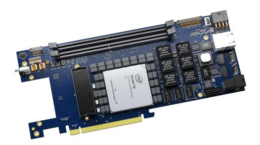
This board also includes the biggest 2800 KLE Stratix 10 density for processing intensive data algorithms hungry for memory depth with its 72GBytes of DDR4. It offers many IOs capabilities with its full High Pin Count(HPC) FMC+ standard connector and the additional board interfaces. The board is PCIe GEN3 x16 capable.
