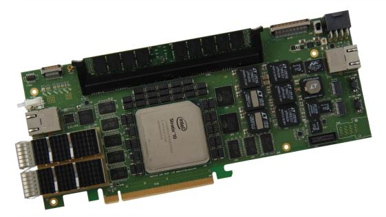
This board includes the biggest 2800 KLE Stratix 10 density for processing intensive and various data algorithms with its mix of memory capabilities in DDR4 and QDR2+. It has an optical interface capability of 200Gbit via two QSFP28 cages and using PCIe gen3 x16. An additional 200Gbit board-to-board interface is provided using a firefly connection.
