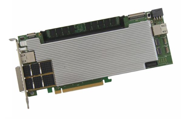
This board includes the biggest 2800 KLE Stratix 10 density for processing intensive and various data algorithms with its mix of memory capabilities in DDR4 and QDR2+. It has an optical interface capability of 200Gbit via two QSFP28 cages and using PCIe gen3 x16. An additional 200Gbit board-to-board interface is provided using a firefly connection. The board is delivered with a custom 1 slot PCIe passive heat-sink.
