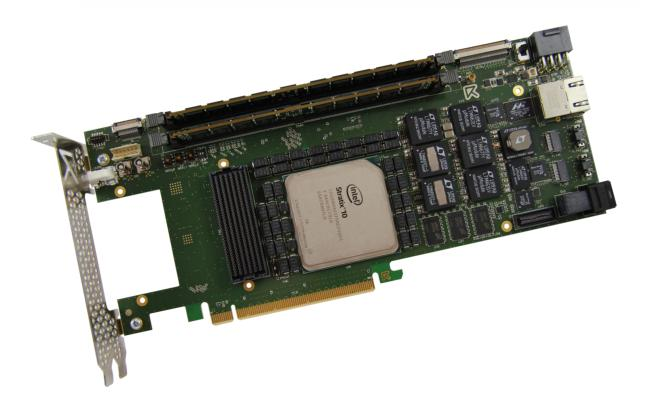
This board also includes the biggest 2800 KLE Stratix 10 density for processing intensive data algorithms hungry for memory depth with its 72GBytes of DDR4. It offers many IOs capabilities with its full High Pin Count (HPC) FMC+ standard connector and the additional board interfaces. The board is PCIe GEN3 x16 capable.
