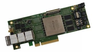
The XpressGXA10-LP1150 features 80G Ethernet, 1 bank of 4GB DDR4, 4 banks of QDR2+ memory, two QSFP+ cages for multi 10GbE/40GbE networking solutions, and 16 transceiver expansion ports.
