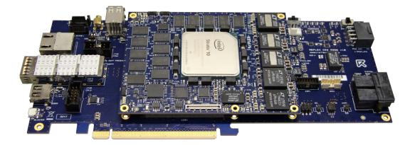
The COMXpress PCIe carrier board is designed to be used quickly in server platform with its PCIe x16 lanes. The carrier board offers several high-speed links like a quad 10 GbE interface with optical front end, PCIe 3.0, SATA3, Mini SAS, USB 3.0.
